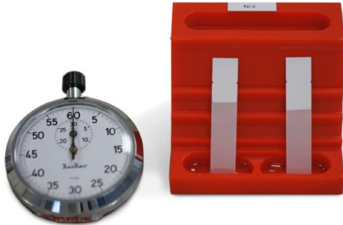
Fig 1. Basic set-up of membrane capillary flow time measurement. Strip width is 1 cm, strip length 4.5 cm, with triangular marks at 4 cm strip length. The time the liquid (water) needs to reach these marks is taken and documented. Water volume is 100 \mu L.
